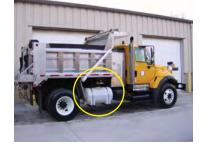
on the side of the dump body. Frame mounted systems are available in 35, 55, 65, and 100 gallon sizes.
