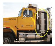
the side of the dump body or between the cab and dump body. Chassis mounted systems are available in 60, 90, 120, and 240 gallon sizes.
